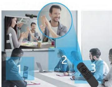
Support Eptz function, 5x digital zoom, electronic pan/tilt movement and digital zoom function can be controlled by remote , support image flip, mirror effect.
